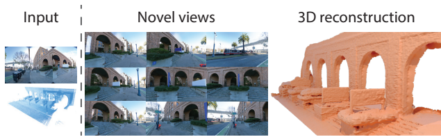
Figure 1. Overview – Given a set of panoramas and lidar observations from an urban setting, we estimate a neural representation that can be used for novel view synthesis and accurate 3D reconstruction.
